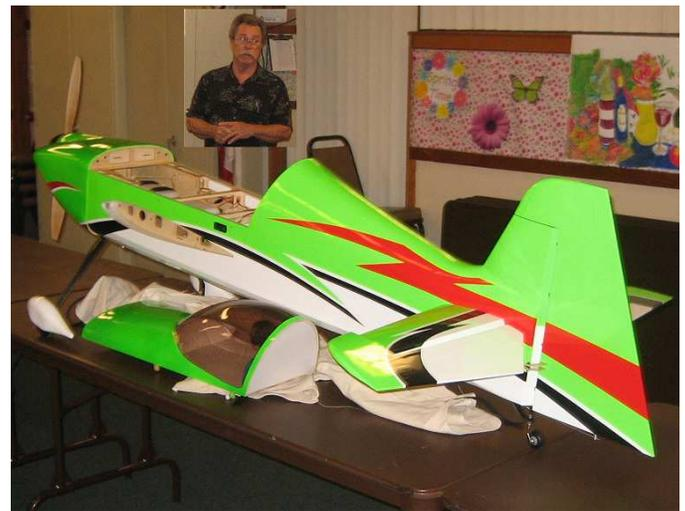
Mel Tufto had an SBACH300. He purchased the model at the AMA show in January. It is powered by a 58DLA motor that generates 6.5hp. He made some modifications as the choke was originally automatic. He changed it so that the choke is manually controlled. The model weights 18lbs when ready to fly. He also purchased a micro-fastener kit, originally priced at \$400 for \$250 as the vendor had only one left as he was packing up to leave. Good Bargain!!
