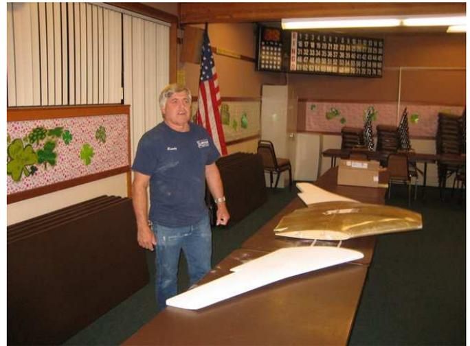
Randy Bronson brought his Beechcraft Starship model. He has completed the center module and the newly constructed wings. He used foam as a “plug” to mold the finished wing. He noted that drywall mud worked well to straighten ripples in the foam. He anticipates using 220cc motors. Electric might be impractical due to the weight of batteries needed to serve the motors. His “win the lottery” power source is turbo prop propulsion. Estimated flying weight is around 30 lbs.
